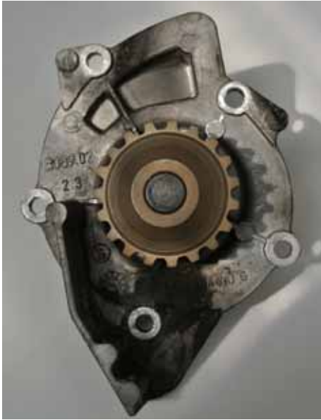
307 HDi water pump showing signs of coolant seepage.
